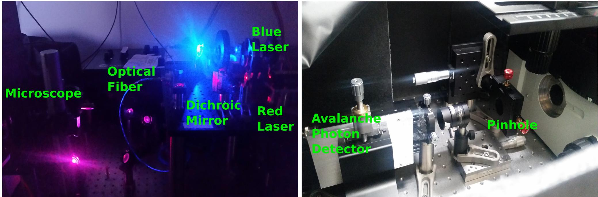
Free to move and rotate Extended observation of freely diffusing molecules (down to 1nm in size) is achieved by monitoring the molecule's position using fluorescence, and applying feedback electric fields after each detected photon to move the molecule back towards the center of the observation volume.
