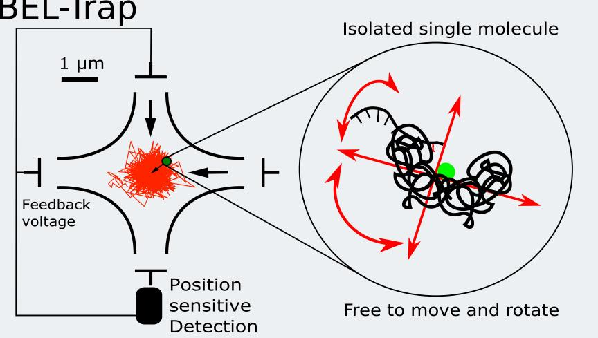
Extended observation of freely diffusing molecules (down to 1nm in size) is achieved by monitoring the molecule's position using fluorescence, and applying feedback electric fields after each detected photon to move the molecule back towards the center of the observation volume.
