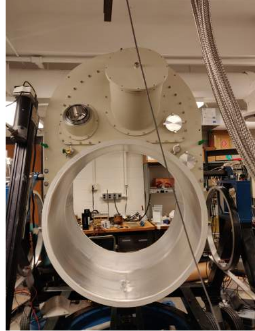
FIG. 1. TSAT outer vacuum chamber displayed in lab with the port on the top left of the image being for the pulse tube that was used in the experiment for this paper
