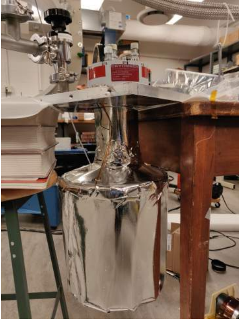
FIG. 7. Experiment setup before adding outer vacuum shell. 30 layers of blankets on the inner cylinder which is the PTC 1 stage
