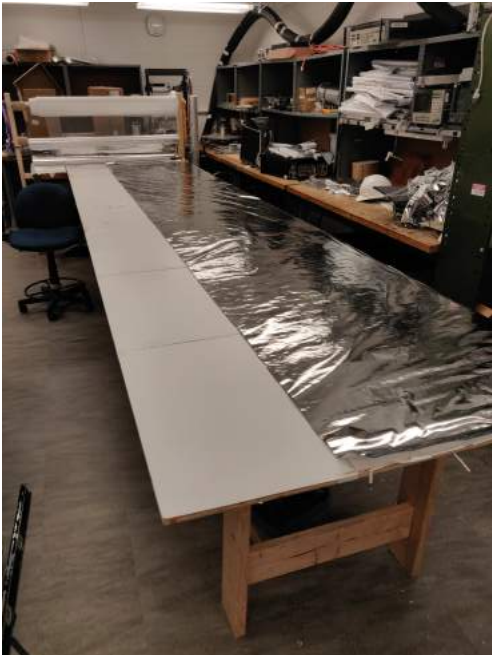
FIG. 4. Table made in the lab with cut MLI for the 40 K stage of TSAT
