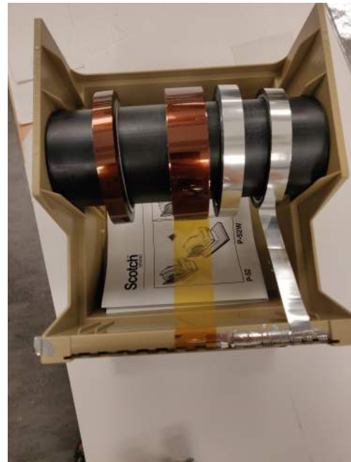
FIG. 5. Tape used in the construction of the MLI blankets. Thin and thick Kapton (left two) and Aluminized Polyester Tape (right)
