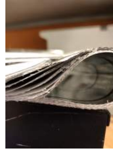
FIG. 8. An example of a 7 layer MLI blanket with the bottom looking normal and the top folded over to show the difference in the individual layers
