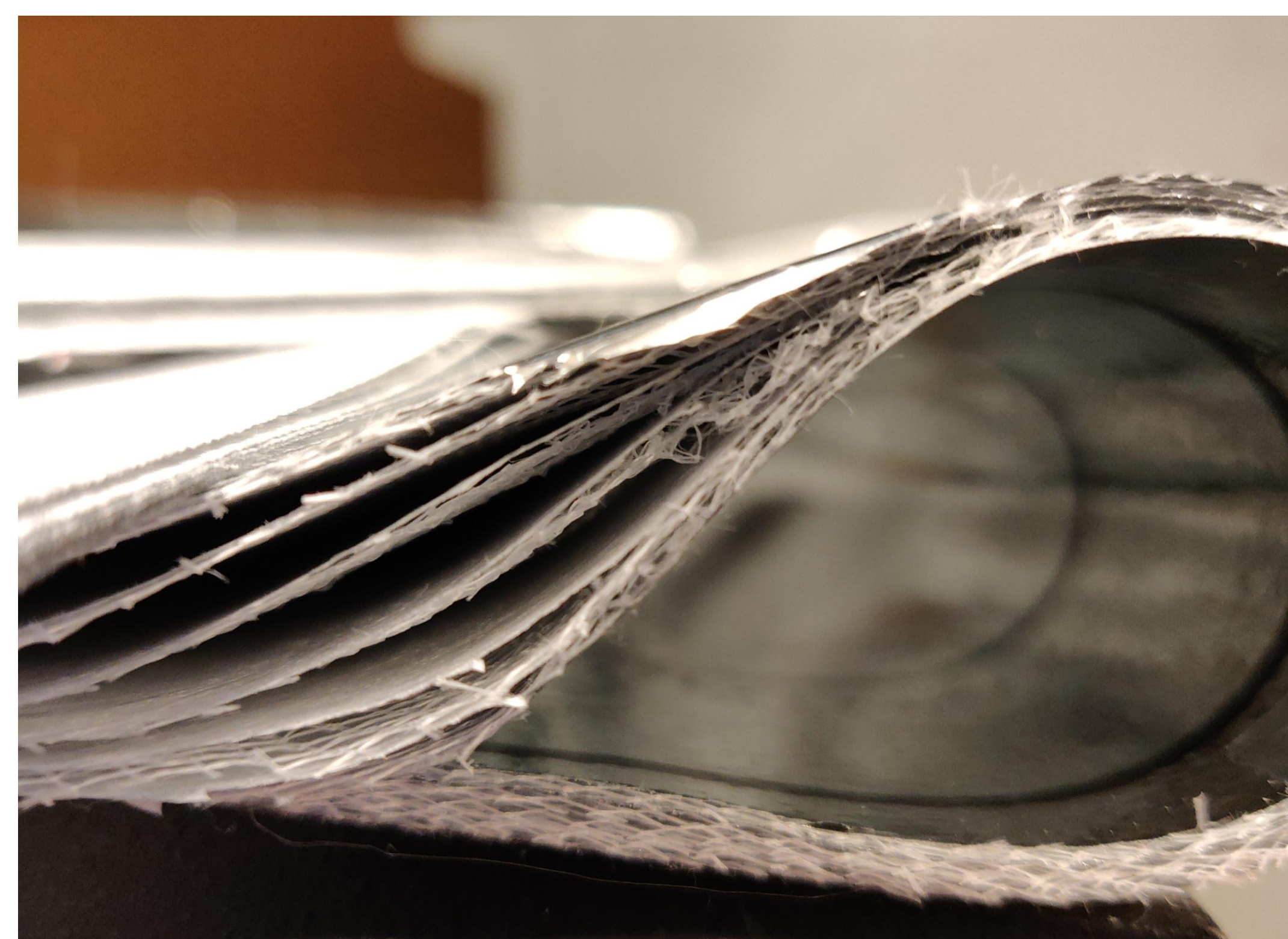
A sample layer of MLI with 7 layers of aluminized mylar.
